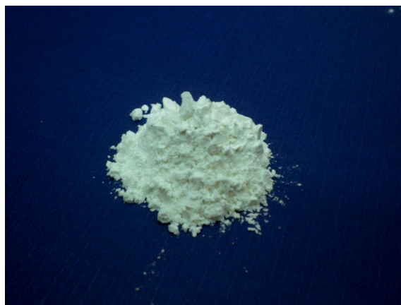
Figure 5.1 – Caustic etch recovery byproduct after filtration and drying
